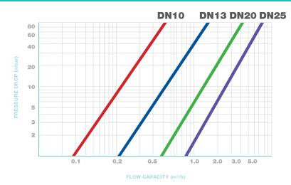
**Schedule 2:** Pressure loss for type of end connection based in internal diameter (DN)
